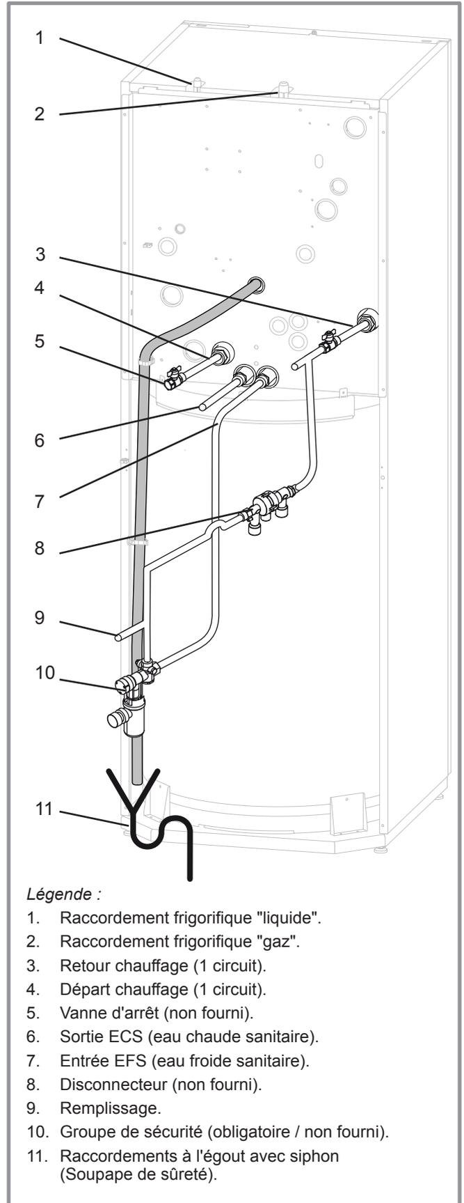
figure 28 - Raccordements
