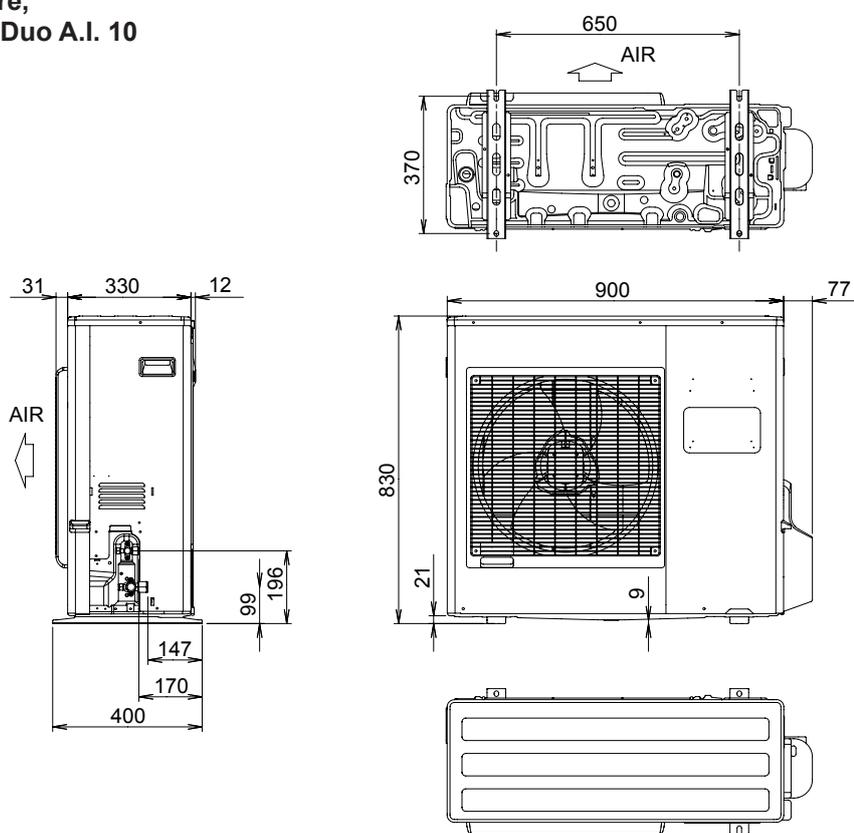
figure 1 - Dimensions en mm
